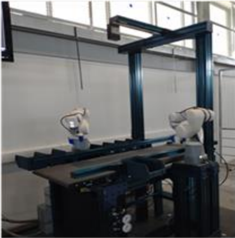
CDW Robotic Separation System
